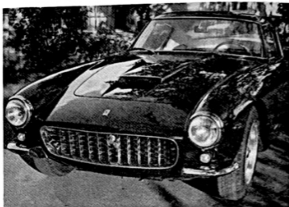
VAUGHN FAMILIE'S 1962 250/GT Ferrari Berlinetta which cost $14,500 new. This brutal looking machine is powered by a 60 degree V-12, developing 300 h.p. at 8,000 r.p.m. out of 180 cu. in. (three litres).
